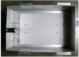
Support grid properly placed in filter pan.
